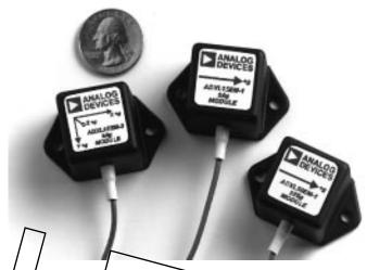
All that is required to use these modules is a +5 volt power supply. The module should be attached (i.e., screwed or glued down) securely to the object being measured, taking care that the axis of sensitivity, indicated by the large arrow on the top of the module, is aligned with the expected acceleration.
